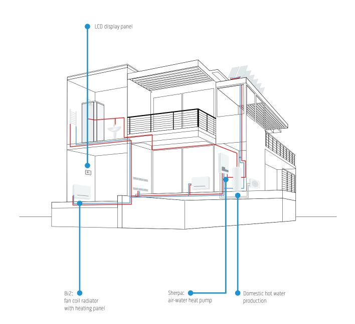
The Aquadue<sup>®</sup> system integrates all OS heat pumps and Bi2 terminals. It also allows the management of potential back-up thermal groups or other elements of the installation, such as circulators. Aquadue<sup>®</sup>Control combines the efficiency of the heat pump inverter systems with the effectiveness of the Bi2 terminals, equipped with DC brushless motor and a radiant heating panel.
